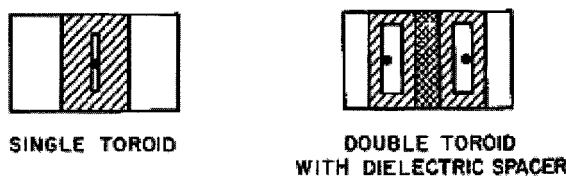
Fig. 9. Single and twin toroid phase shifters (from [141]).
